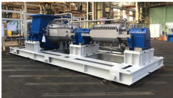
Partanna Steam Turbine during final assembly
